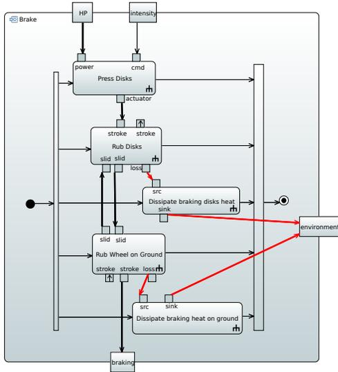
Fig. 1. Excerpt of the functional architecture of the Braking System
